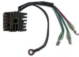
Universal 3 Wire Rectifier Fits Various Motors 6-300hp Wires: Green, Green/ Green/White, Red, Black (Earth) Replaces 8109397M, 6F5-81970-62, 664-81970-62, 664-81970-61 Part No: 676-81970-00
