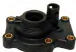
Pump Housing W/ Brass Bushing 20, 25, 35 HP W/ Thru-Prop Exhaust Part No: 393632
