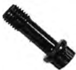
Torque Spec 30 ft. lbs. plus 90 Degrees
