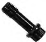
Torque Spec 30 ft. lbs. plus 90 Degrees
