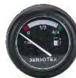
Fuel Gauge 30-240 OHMS 12/24 volts Hole size 52mm Part No: VP40110 (Black) Part No: VP40110W (White)
