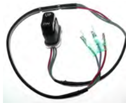
Wiring Harness ONLY With 2 relays Converts 2 Wire Trim motors for use on older 3 wire systems Part No: 8268
