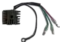
Universal 3 Wire Rectifier Fits Various Motors 6-300hp Wires: Green, Green/White, Red, Black(Earth) All approx. 150mm long Unit approx. 40 x 35mm 1 Centre Mount Hole Part No: 6F5-81970-62
