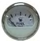
Fuel Gauge 0-180 OHMS 12 volts Hole size 52mm Part No: VP86130
